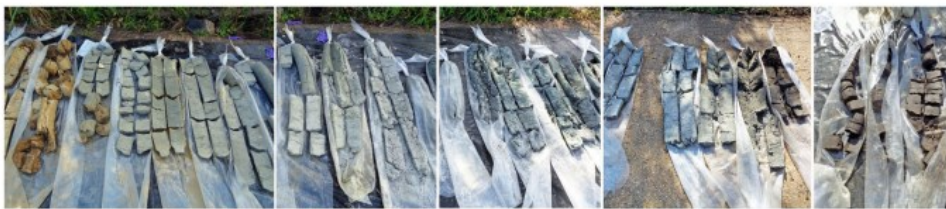
Figure 5. The core, from left to right, penetrated the brown weathered Yazoo Clay, the gray unweathered Yazoo Clay (frame 1), the sandy Moodys Branch Formation (2-4), and the Cockfield Formation (4-5) with a lignite seam at the top (4, last core at right).
