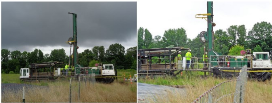
Figure 4. Sonic drilling rig coring at the Southeastern Wood Preserving Superfund Site on June 19, 2017, in stormy and fair weather.
