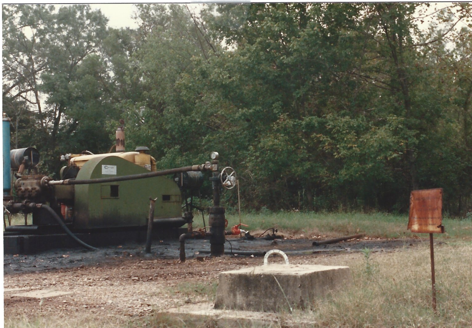
Photo 4: Union Producing #1 George Woodruff, the discovery well for Tinsley Field. As of the date of this field trip the well was being used for water injection for secondary recovery operations.
