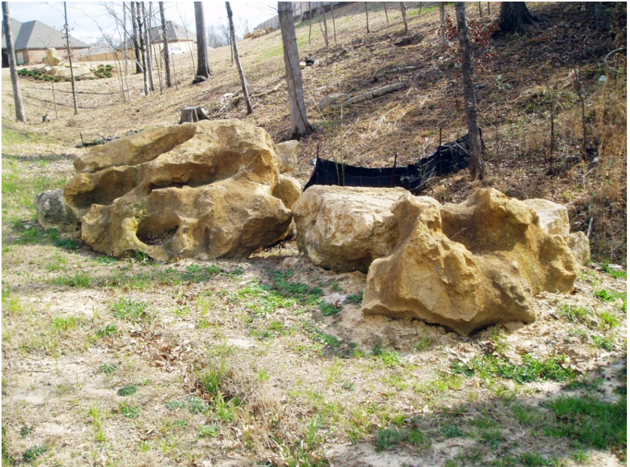
Figure 4. Boulders of Glendon Limestone excavated at the Bruenburg Subdivision in western Clinton, Mississippi, next to the salamander crossing on the Natchez Trace Parkway. Karst cavities can be seen in the limestone. Picture courtesy of Tom Mann.
